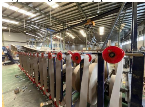
Figure 8 Winding Process with Large Diameter Raw Materials
