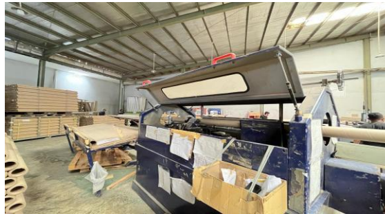
Figure 9. Winding process with raw materials of large diameter 2
