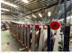
Figure 8 Winding Process with Large Diameter Raw Materials
